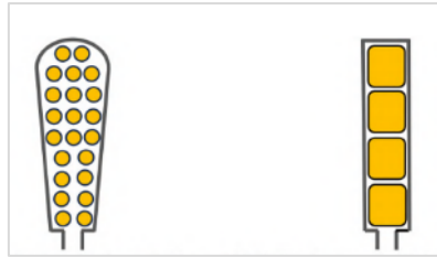
Figure 11 Conductors for Random Winding and Hairpin Winding [16]
